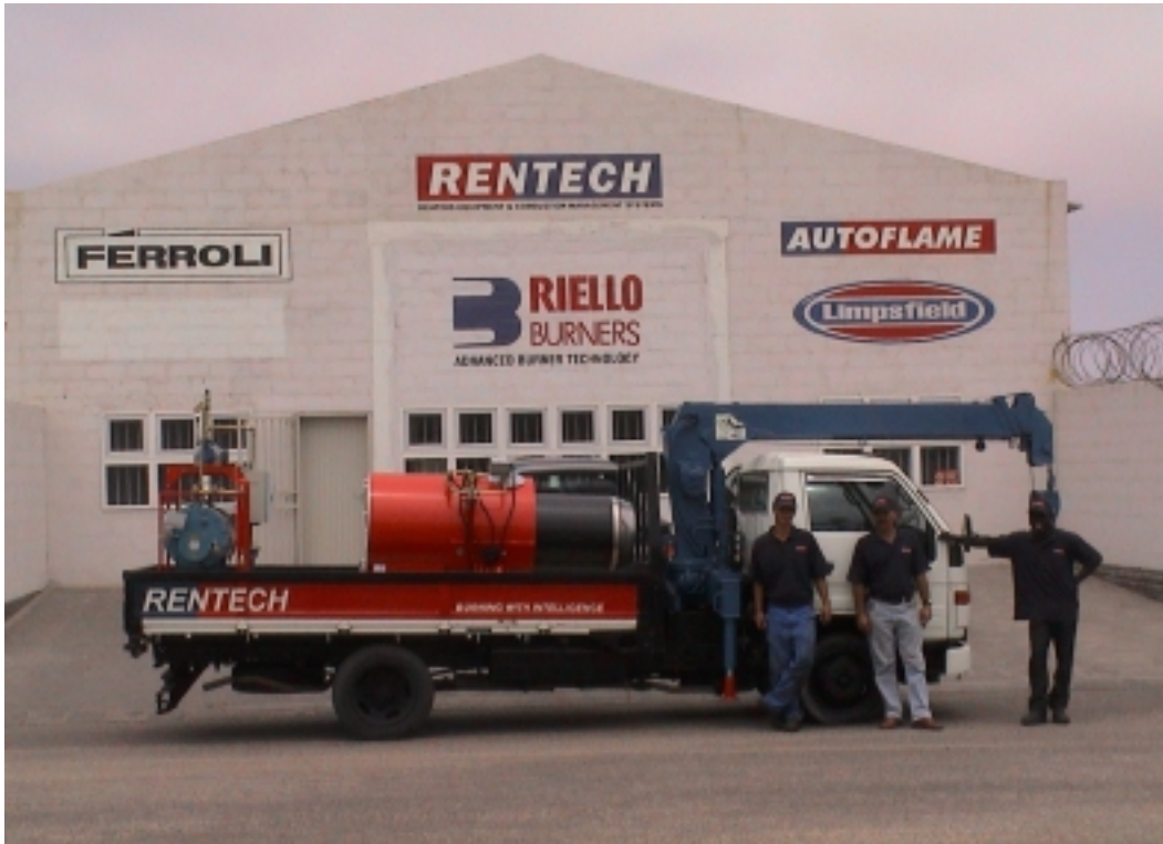
18 Ton boiler burner and pump skid ready to be delivered to site
