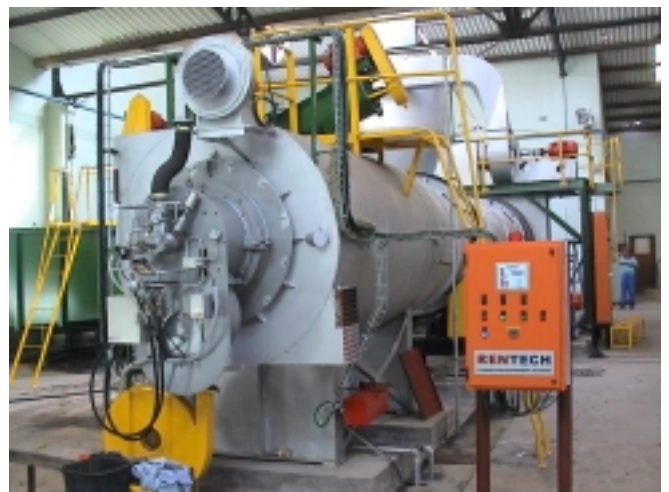
Burner after refit and conversion to Autoflame
